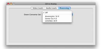
The Processing pane provides down conversion options for Mini Converter SDI to Analog and Mini Converter HDMI to SDI.
