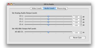
In the Audio Levels pane, the four analog audio channels can be adjusted independently as analog audio levels may vary between channels because analog is not perfect. However the 8 channels of AES/EBU digital audio are all adjusted together as digital audio levels will not vary between channels and so should all be raised or lowered together.
