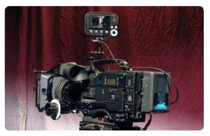
Remove the drive from the sideKick HD to hand off to post-production for straight to edit workflow.
