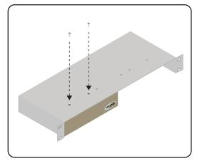
$\textbf{Step 6} \quad \textbf{Unit has been installed into rack tray}.$
