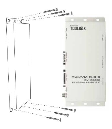
The GefenToolBox DVIKVM ELR Sender and Receiver may be mounted vertically in a wall or cabinet with wood/drywall screws as shown in the diagram above. There should be an inch or two of clearance between the edges of the unit and any walls or vertical surfaces to allow for enough clearance for insertion and retraction of cables at the DVI and RS-232 connectors.
