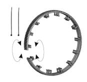
USE SMALL ZIP TIES FOR TEMPORARY ATTACHMENT OF THE LENS GEAR
